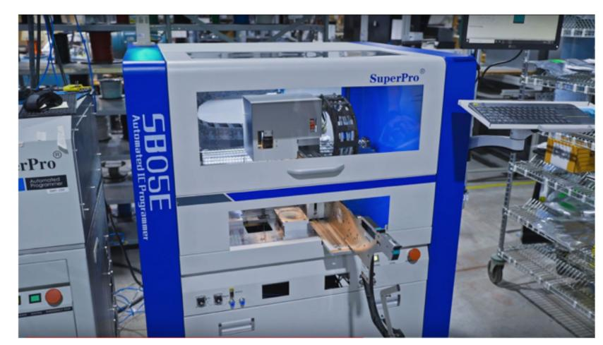
Z-AXIS has upgraded its robotic IC programmer to increase processing speed and reliably program the latest fine-pitch processor and flash memory packages.
